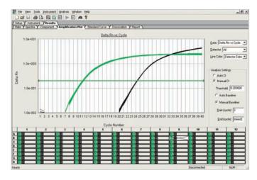
Multiplexed TaqMan® assays on the 7300 System showing amplification of cDNA (96 samples) using probes labeled with VIC® (green) and FAM™ (black) reporters for the 18S and TGF-beta target sequences, respectively.
