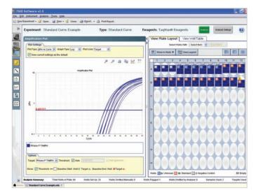
Amplification plot from a 7500 Fast system above shows results from a TaqMan Fast RNAse P Instrument Verification Plate. Using this assay, the 7500 Fast platform can distinguish between samples containing 5,000 copies and 10,000 DNA template copies respectively, with a statistical confidence level of 99.7% and a run time of about 30 minutes.
