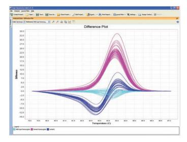
Difference plot generated by Applied Biosystems' HRM Software. A 96 bp-long fragment of the human Keratin 23 gene containing a G>A variant was amplified from DNA samples and melted on the 7500 Fast System. Three replicates of each genotype are shown, wild-type homozygote A/A (green), variant homozygote G/G (red), and heterozygote G/A (blue).
