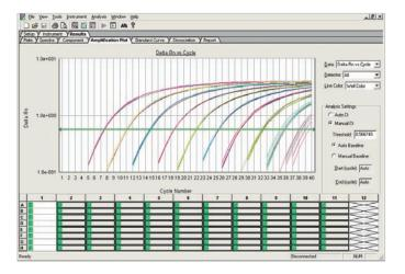
Log of change in normalized reporter fluorescence plotted against PCR cycle number. This plot from the 7300 System illustrates 9 logs of linear dynamic range for a TaqMan® assay of plasmid DNA containing the hCCNB1 target sequence in tenfold serial dilutions (hCCNB1 is human g2/mitotic specific cyclin b1, chromosome 5, 5q12).
