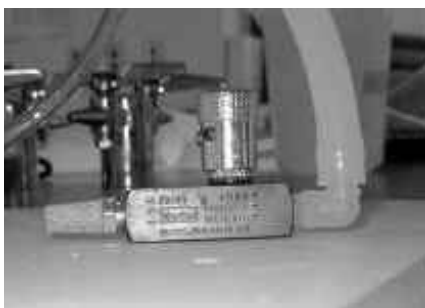
Fig. 22. Gold vacuum control valve.
