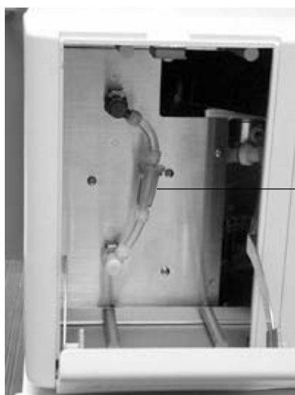
Fig. 3A. Sheath filter internal fluidics features.
