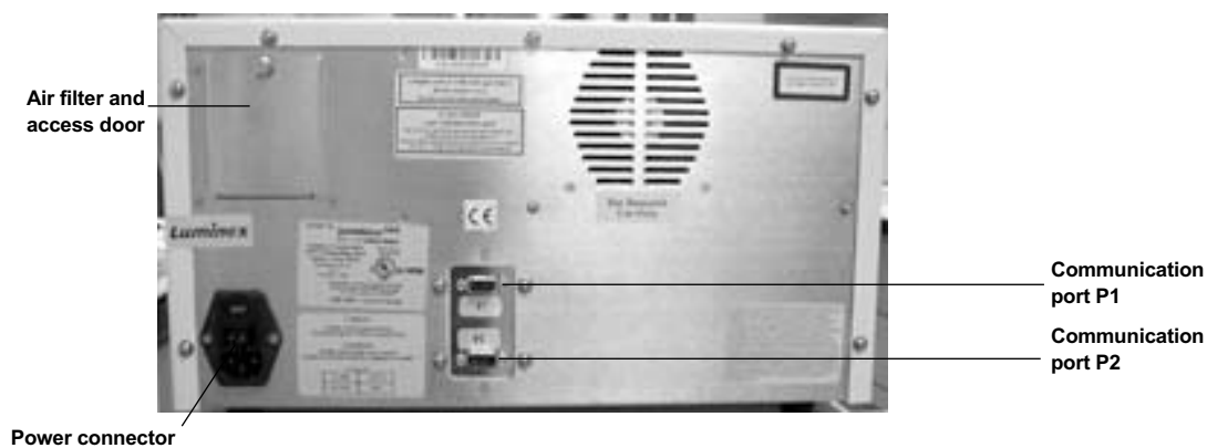
Fig. 2. Array reader – rear panel features.
