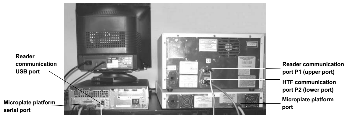
Fig. 11. Completed connections of computer and monitor to the Bio-Plex suspension array system.
