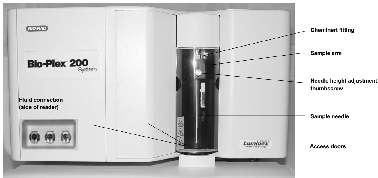
Fig. 1. Array reader – front and side panel features.
