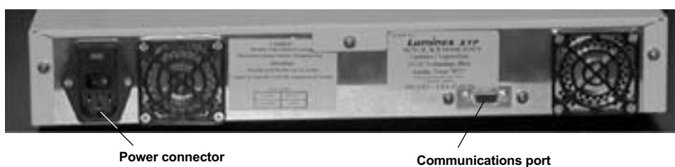
Fig. 5. Microplate platform – back panel view.
